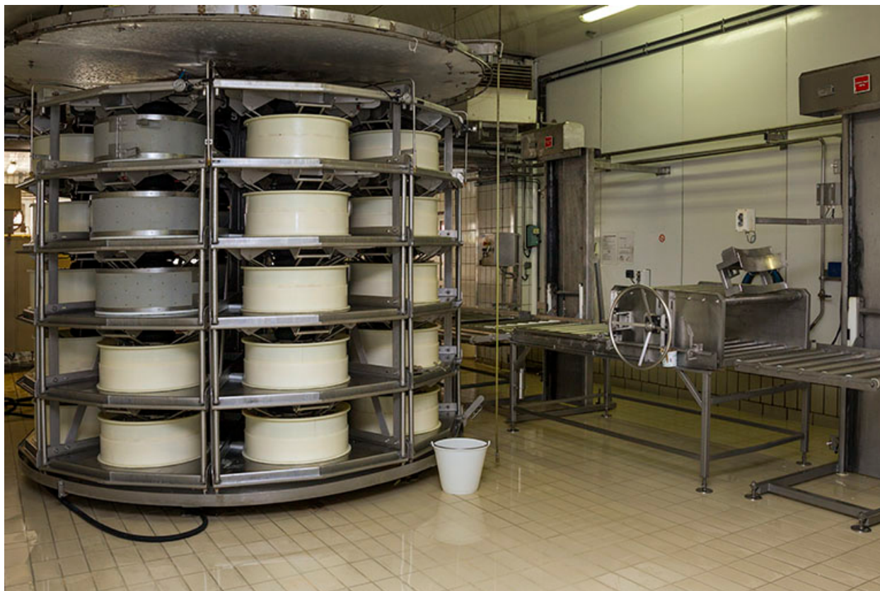
Installation de pressage.
