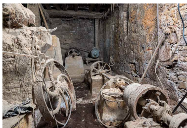
Atelier de fabrication, sciurier : transmission de la turbine. Phot. Sonia Dourlot IVR43_20172501701NUC4A
