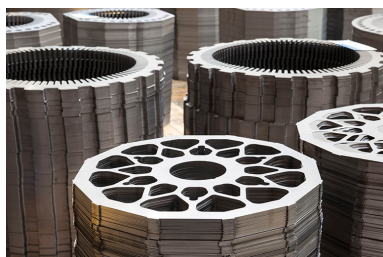
Plaques de stator. Phot. Jérôme Mongreville IVR43_20162500189NUC4A
