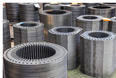
Plaques de stator. Phot. Jérôme Mongreville IVR43_20162500188NUC4A
