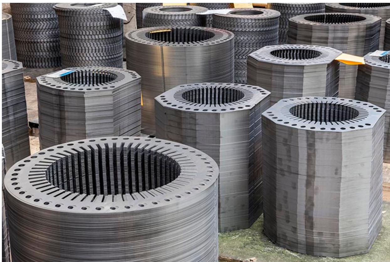
Plaques de stator.
