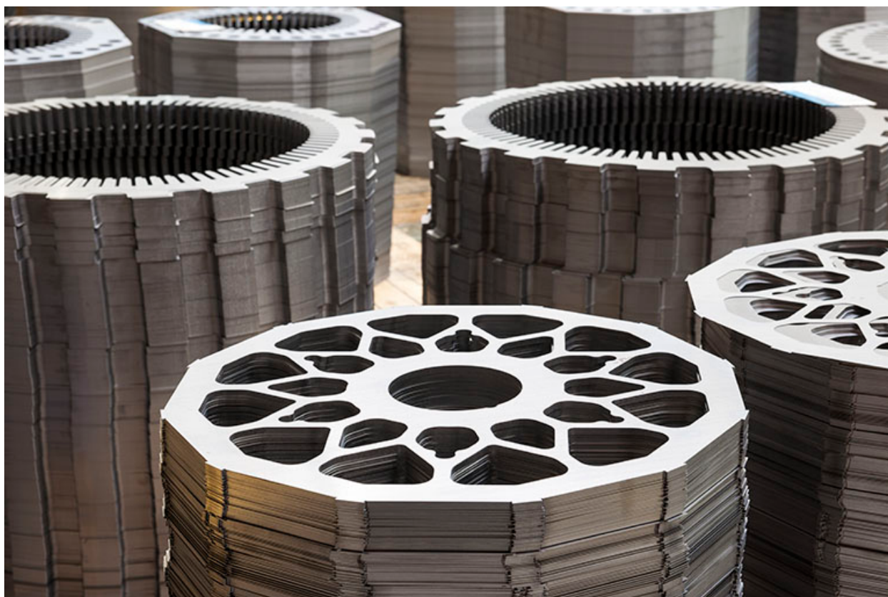
Plaques de stator.
