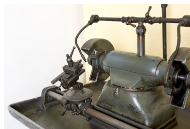
Porte-outil et poupée mobile. Phot. Sonia Dourlot IVR43_20162500476NUC4A
