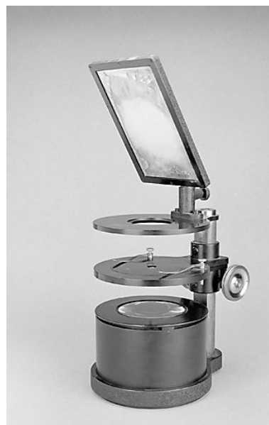
Epidiascope with appliances adapted for Micro-projection. Projection without Ocular,
