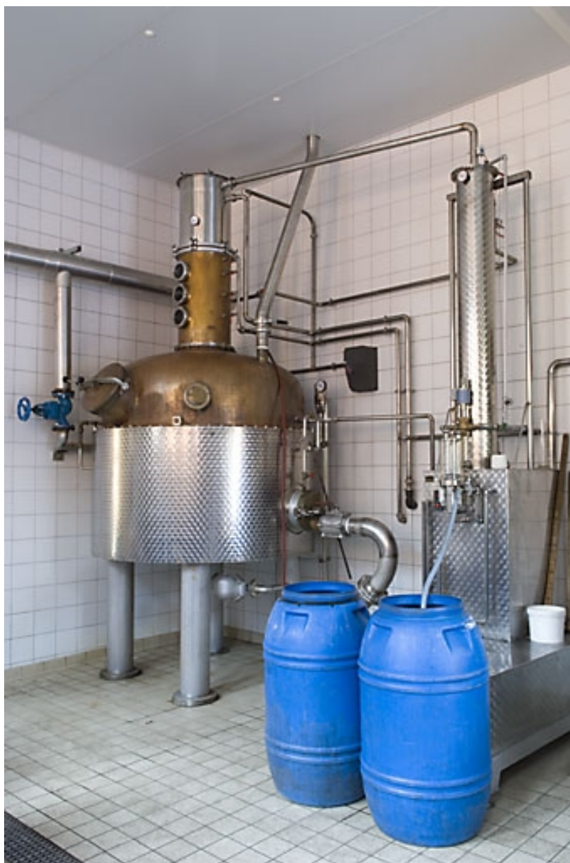
Atelier de distillation. Alambic Arnold Hosstein.
