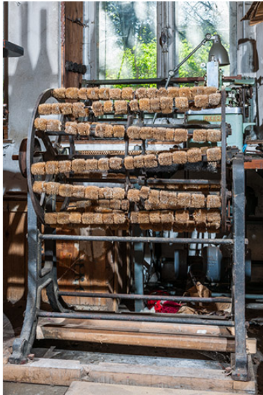
Machine à carder rotative. Phot. Jérôme Mongreville IVR43_20142500227NUC4A
