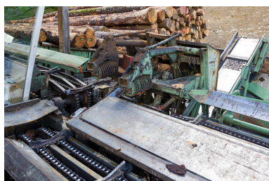
Installation de billonnage. Phot. Yves Sancey IVR43_20132501748NUC2A
